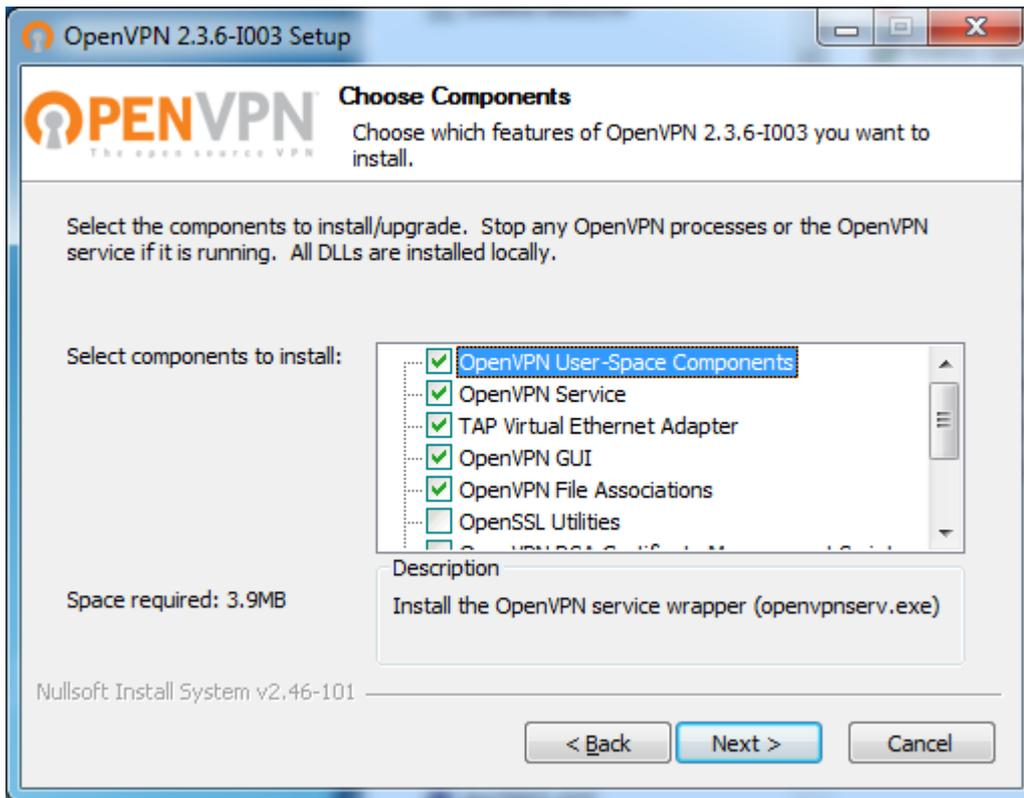
During the installation an additional network interface is installed. The appearing notification offers the options „install“ and „not install“, you need to select „install“ or the OpenVPN client won't work.
