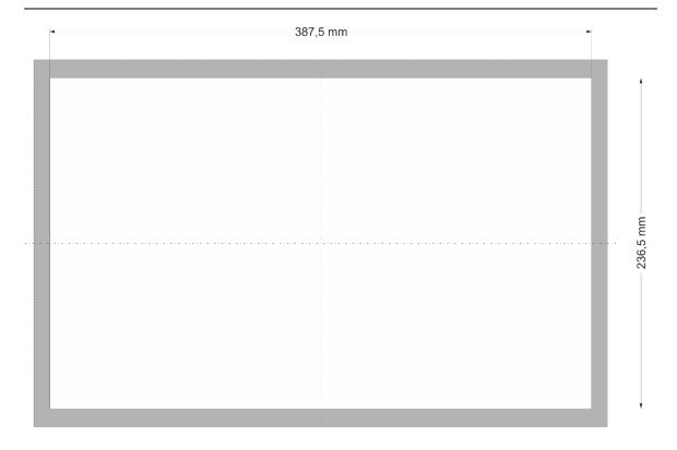
Fig. 8: DC-Pi Prime 15 mounting cut-out
