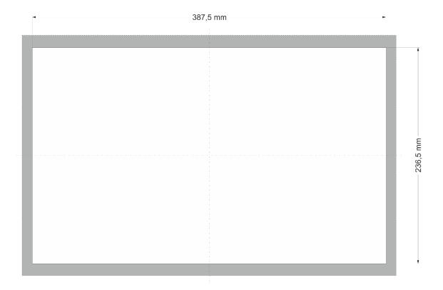
Fig. 8: DC-Pi Prime Open 15 mounting cut-out
