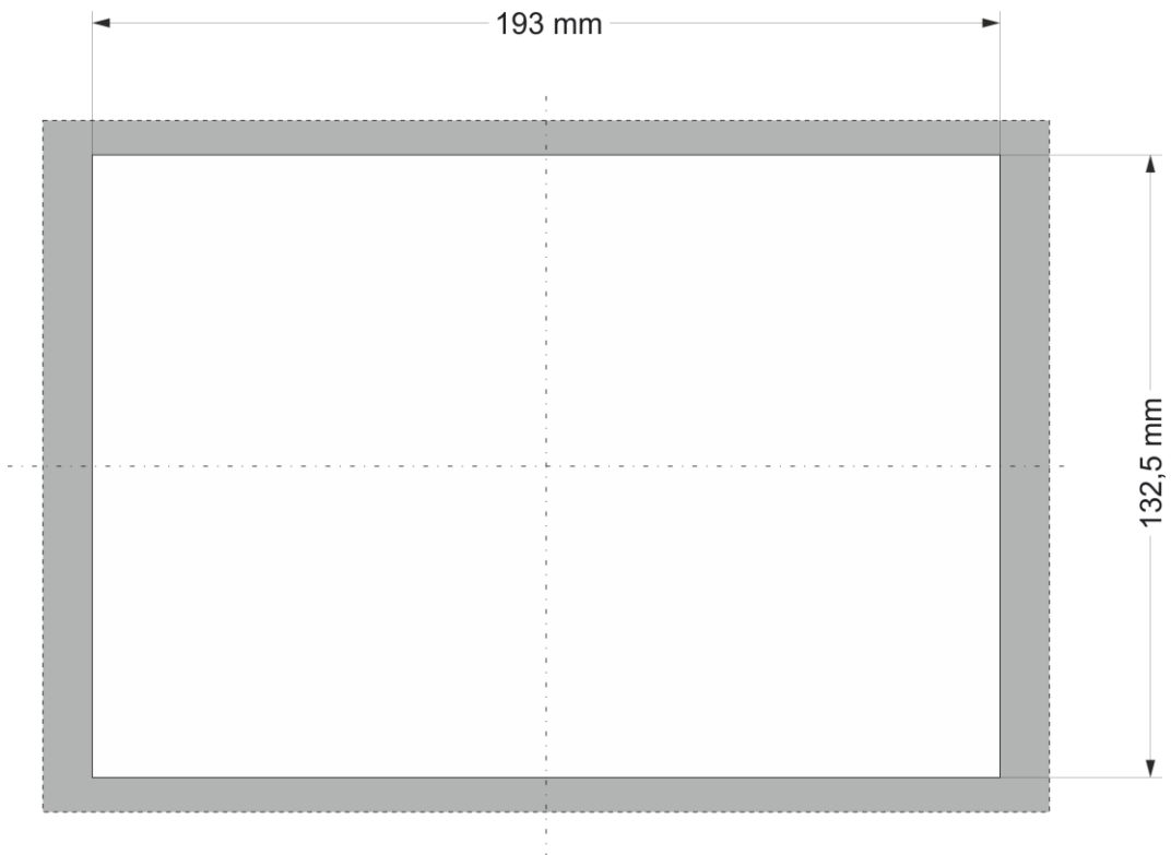
Fig.3 : Installation cutout ET-Pi Prime 7
