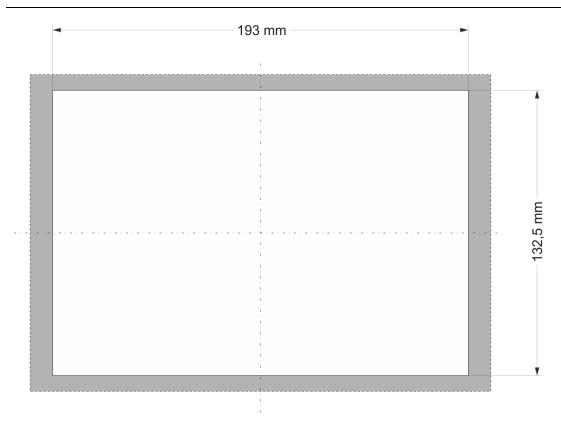
Fig.3 : Installation cutout ET-Pi Prime 7
