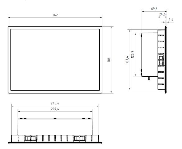
Fig.4 : Dimensions ET-Pi Prime 10
