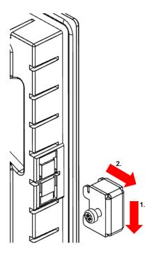
Fig.27: Removing the clamping brackets
