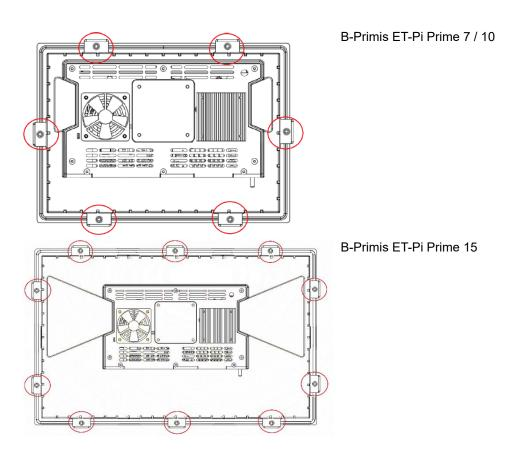
Fig.26: Loosening screws
