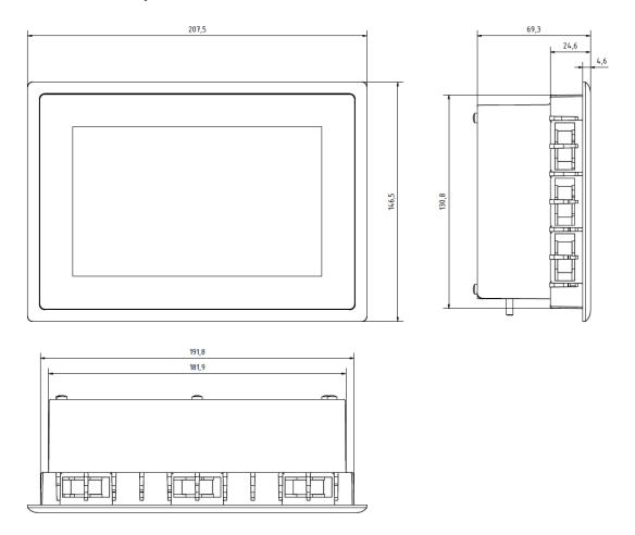
Fig.2: Dimensions ET-Pi Prime 7
