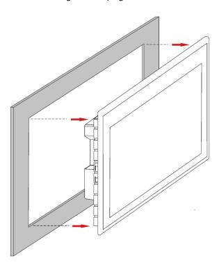
Fig.28 : Sliding the device out of the mounting cutout
