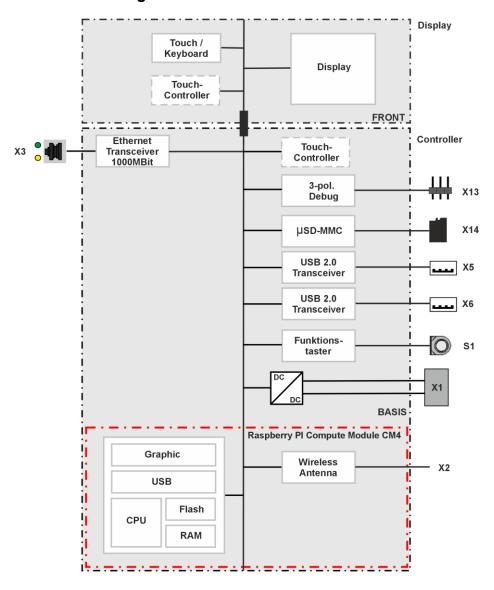
Fig.10: Block diagram ET-Pi Prime
