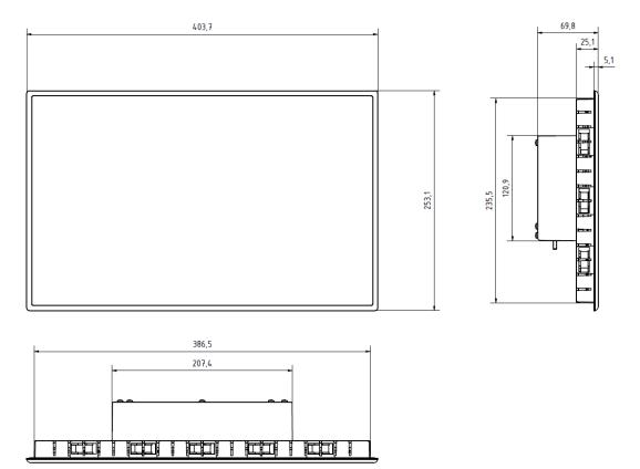
Fig.6: Dimensions ET-Pi Prime 15
