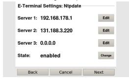
Fig.17: NTP settings of the device
