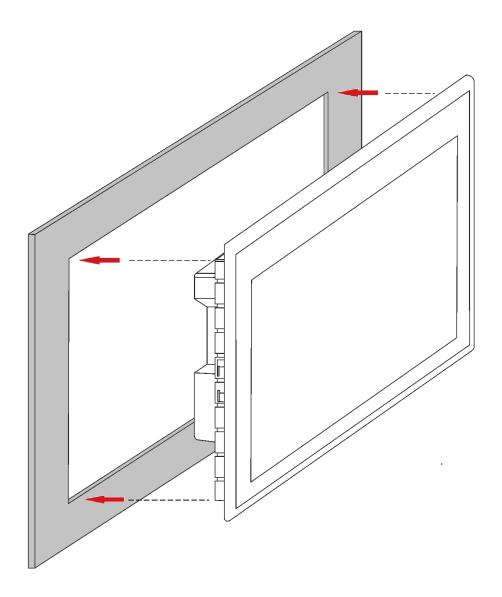
Fig.8: Insertion into mounting cutout
